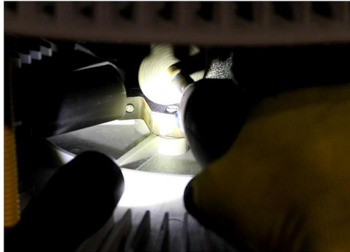
4. Turn on the vacuum and position it to the left while holding the running Dremel from the right as shown.
