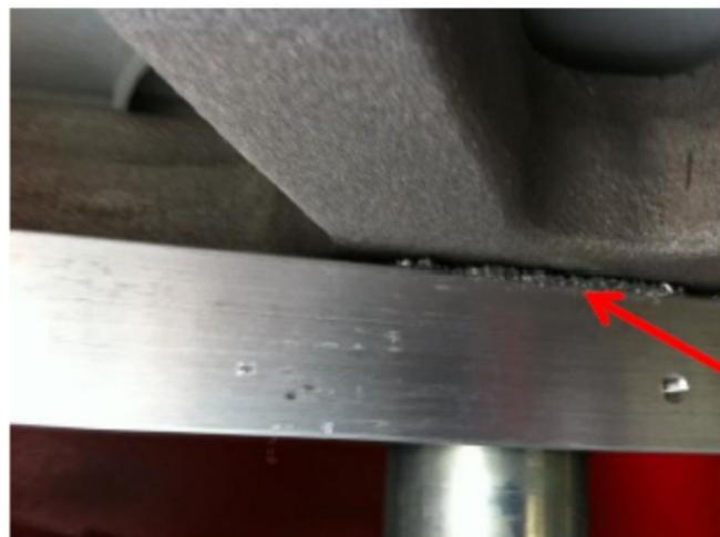
1. Shavings on the top of lower crossbeam indicate that the bolts are grinding and the shavings will likely have done damage to the lower drum bearing
