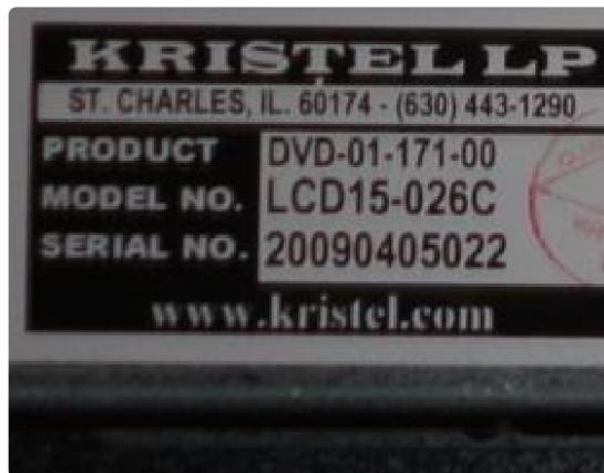
When installing a new touch screen or reinstalling software for an existing touch screen, first determine the model of touch screen you are using. The touch screen model number is located on
