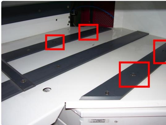
Remove the four screws holding in the QLM bay. These screws are shown within the red boxes on the left. This requires the 5/32" Hex Head Driver.
