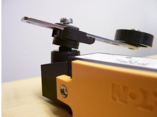
This picture illustrates the toggle bar as it is very close to being removed from the rest of the sensor. At this point, the toggle bar can be removed and then reset to the position that is needed to properly identify the status of the QLM case.
