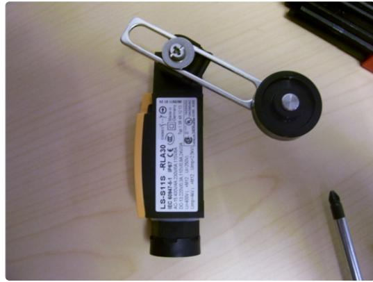
This picture shows the correct neutral position of the presence sensor. Set the toggle bar as close to this position as possible, and then tighten the screw.
