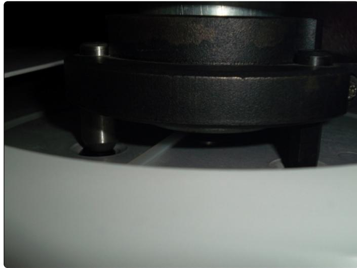
Once the QLM is engaged, align the 3 prongs on the QLM hub with the 3 holes on the QLM.
