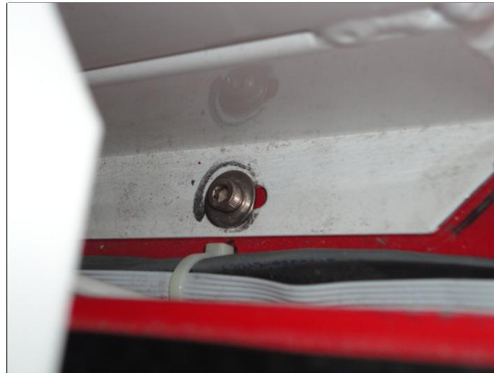
1. There are two bolts in the front of the QLM Bay that secure it to the bottom of the kiosk. One on either side as pictured to the left.
