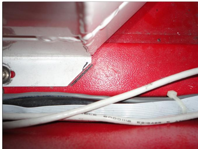
3. After verifying, it is good practice to mark with a sharpie the front edge of the QLM Bay's position. If it slips out of place, a future adjustment is much easier.
