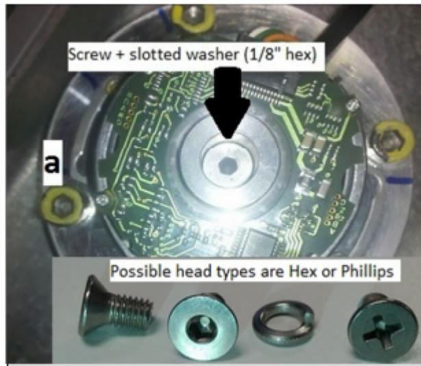
(a) Disengage the encoder locking screw and washer using a 1/8" hex or a short Phillips head screwdriver. Sometimes you can just loosen this screw without removing it. When it is loose, the encoder is able to flex up and down on its mount and should slide right off the top of the shaft. If you remove the screw entirely, don't worry. Just don't lose the screw and washer – both parts are critical.
