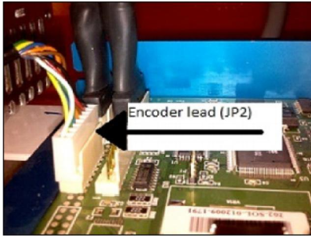
3) Plug the lead from the encoder into the J2 slot on the Arcus board. It is on the left side, in front of the X Amp connection. It is keyed and should only fit one way. To be sure, the white wire is closest to the front of the board, the black wire towards the back of the board.
