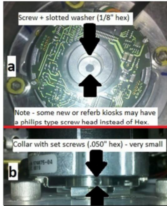
3) Loosen the encoder from the drum's vertical shaft. This will be done one of two ways:
