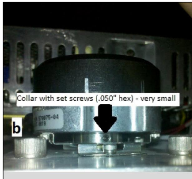
(b) Alternatively, there may be a locking collar on the encoder and glue in the center. The set screws (usually two) need to be loosened to disengage the center shaft. Once loosened, the encoder must be pried off with great force to break the bonds of the glue/Loctite that is used on the shaft. After it is removed, clean the center shaft, glue residue will inhibit a new encoder from being installed.
