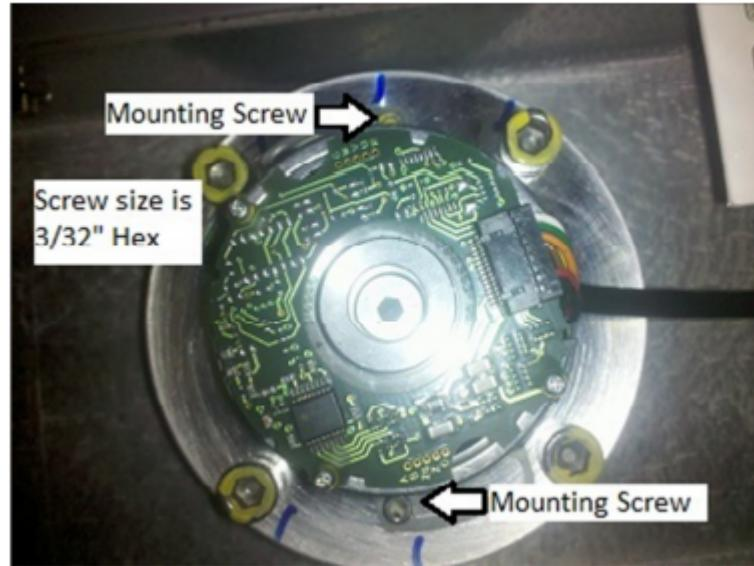
2) Remove the mounting screws on either side of the encoder using your 3/32" hex tool. Don't lose them, they are small. The encoder may now rotate a bit, but it is not free. The connection between center axel and encoder must be loosened.
