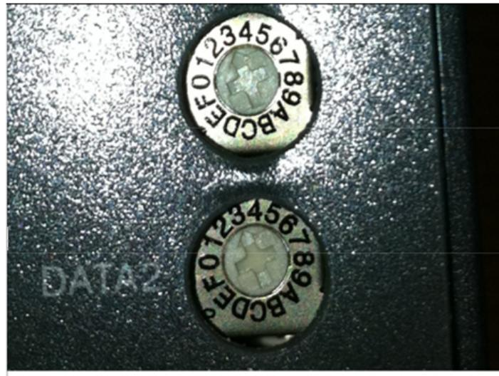
On the Y-amp (top amplifier), we will turn the dials on data 1 and 2 by turning the screw to the right 3 clicks so that the arrow is pointing on 3.
