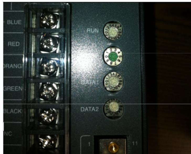
We will now adjust both data 1 and 2 on the Y and X amps. They are both currently set to 0. Remember, it is very important that this be done with the power to the machine off!
