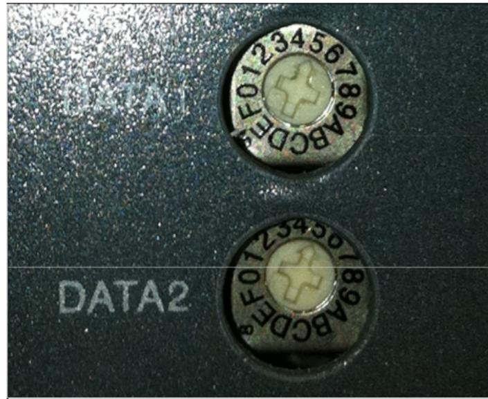
On the X-amp (bottom amplifier), we will turn the dials on data 1 and 2 by turning the screw to the right 5 clicks so that the arrow is pointing on 5.
