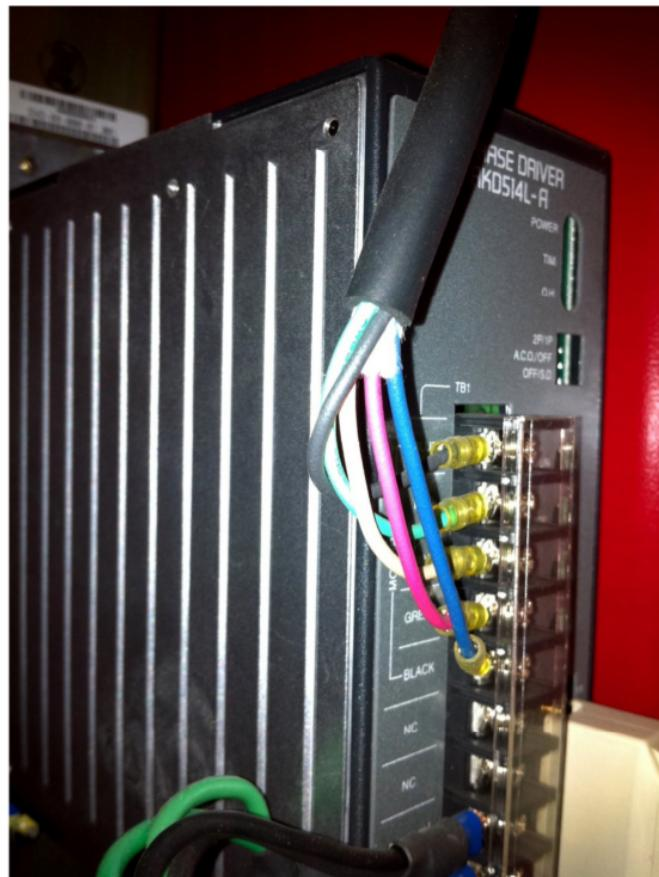
**1. Power Down the Machine and disconnect the Motor Driver Cable from the UPS.**
