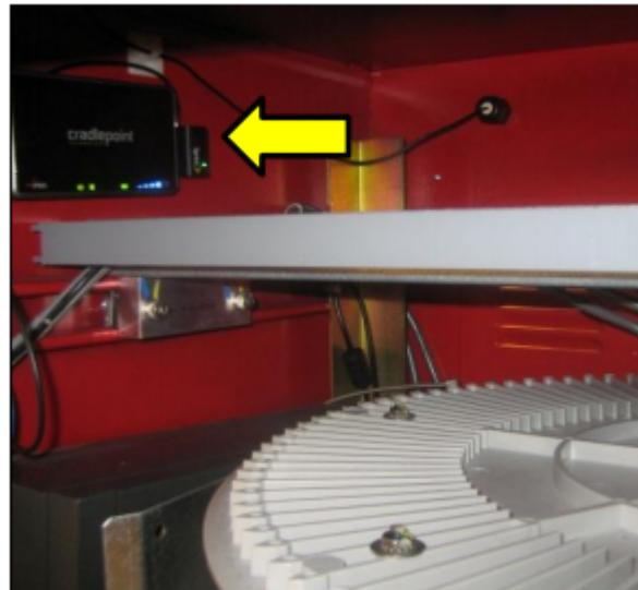
2. While looking inside the machine, look for an opening in the upper rear corner of the kiosk to feed the antenna through. If none is found, drill a hole with a unibit and an electric drill to run the antenna cable through.
