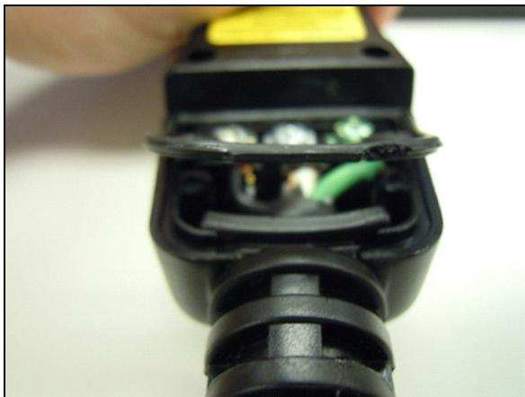
Lift the gasket and pull the cable out of the GFI.
