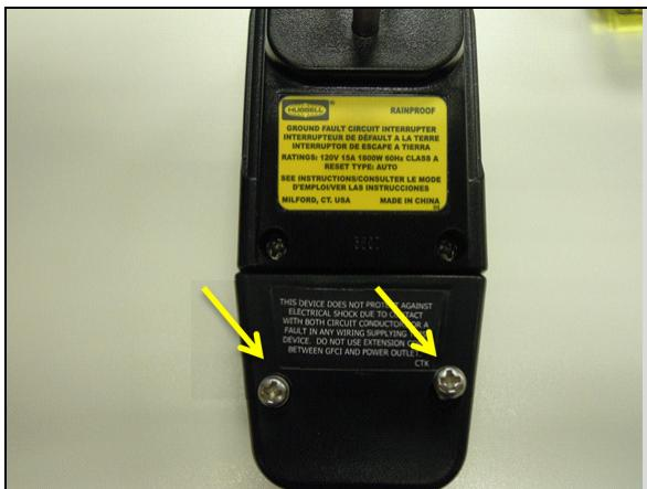
Remove the bottom plate by removing the 2 screws located as indicated by the arrows.
