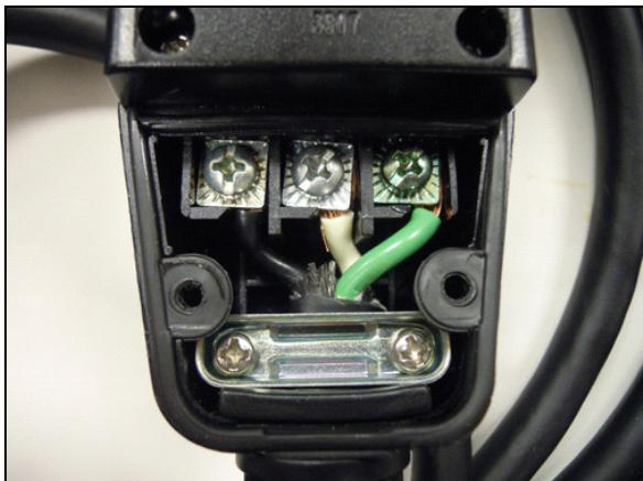
Secure the cable by placing the bare wire into the terminal and tightening the screw down.
