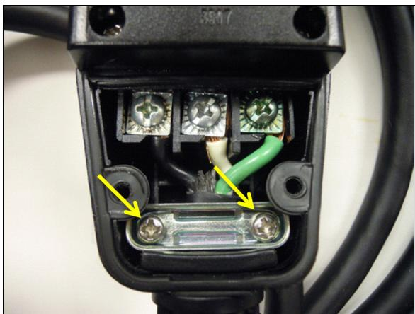
Loosen the two screws holding down the main cable clamp.
