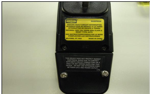
Replace the cover and tighten the screws.
