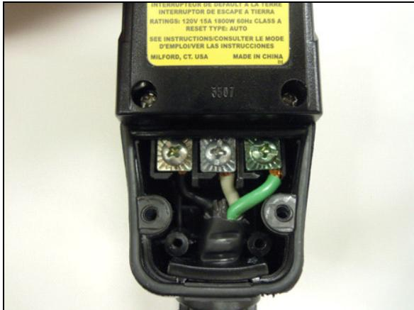
With the cable free you can place it into the new GFI. Note: If needed, you can loosen the terminal screws to make inserting the wires easier.
