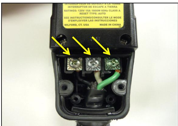
Loosen the 3 terminal screws holding each wire in. Note: Remember the color pattern. Black (left – hot), White (middle – neutral), Green (right – ground).
