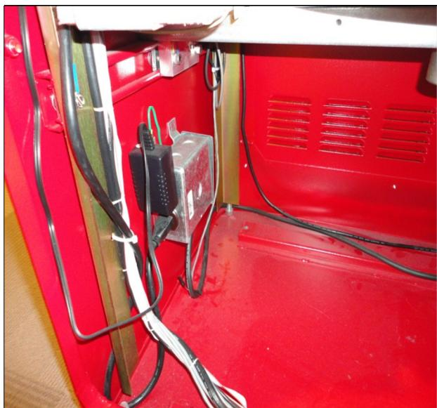
10. Outlet box -Have the electrician take apart the plug box to the left of the QLM and make sure it's wired correctly and all the wires are tight – this has been found to be the cause a couple of times and should be followed up by testing the wiring with a line tester.
