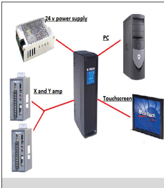
There are 4 components plugged into the Back up Battery:
