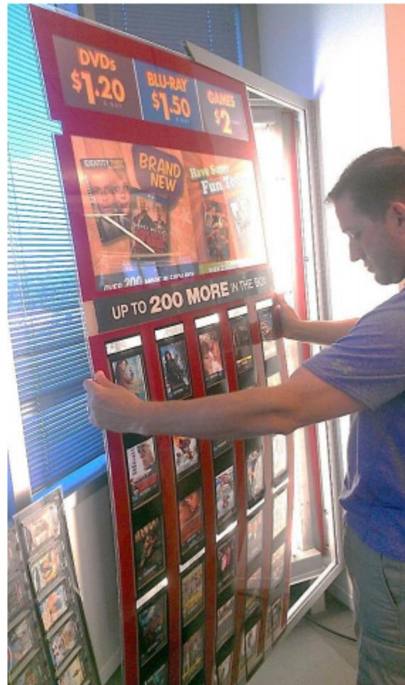
4. Once removed, insert the new Plexiglass into position. It may be easier to place the bottom half of the Plexiglass in first; slightly bend and insert the top half into
