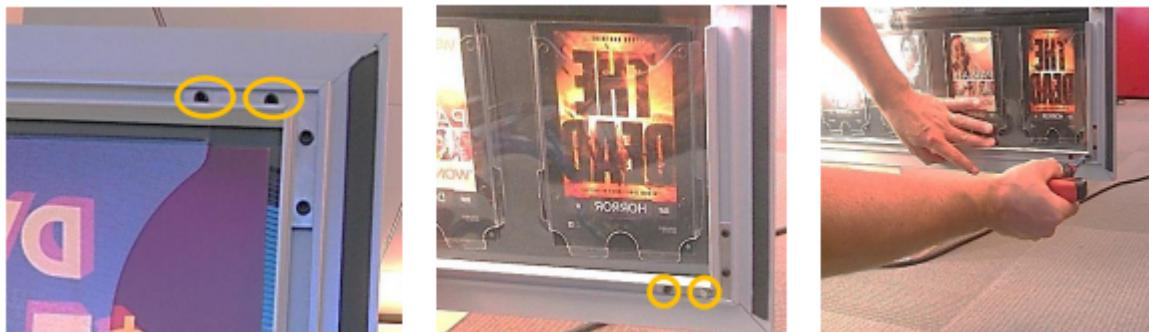
2. Loosen a set screw located on the top left hand corner of the light box door using a nut driver. The picture below identifies the correct screw to loosen.
