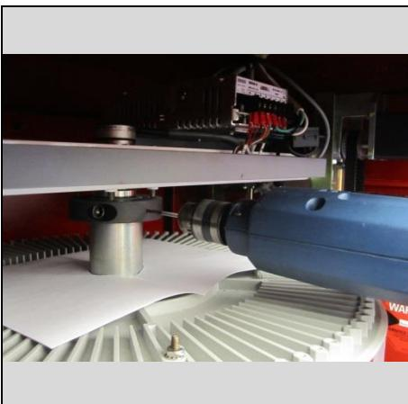
Use # 29 drill bit to make the hole, Drill hole through the smaller center hole on collar jig to line up with shaft.
