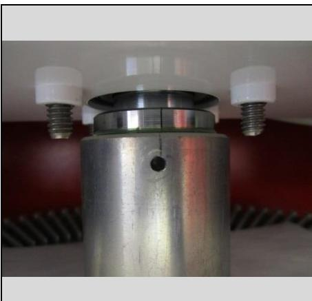
Remove Collar Jig & clean up the shaft.
