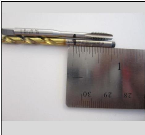
Tap the threads to 0.75"; you can mark the tap with sharpie to make sure.
