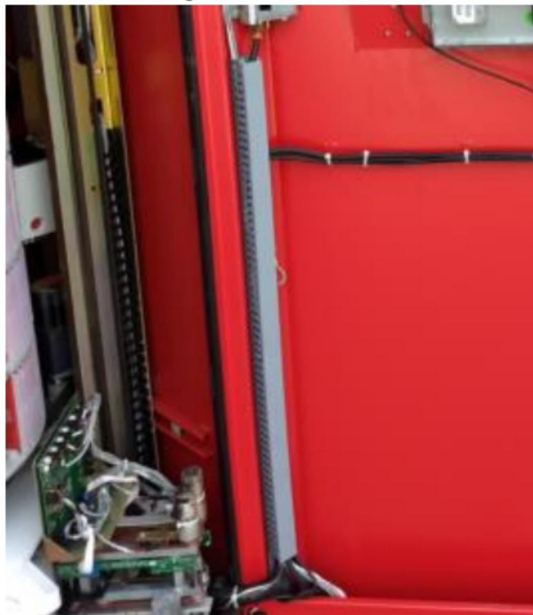
11. Depending on whether the wire tie is above or below the motor wiring connector, cut the wire tie securing the VD motor wiring to the motor housing. The below pic shows the wire tie on the motor-side of the connection and it does not need to be cut. Occasionally, the tie is on the kiosk-side of the connector and must be cut.
